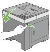
5 Open the belt unit until it stops and remove the jammed paper. Confirm that there are no scraps of paper remaining inside the printer.
